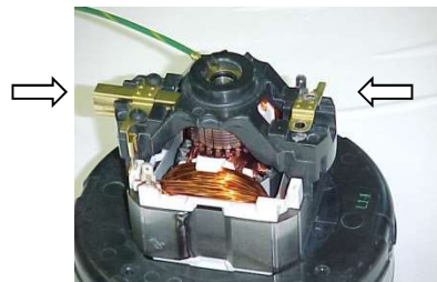
Fig 2: 1 Motor Brush Removed
